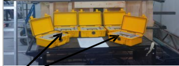
pressure cells reading 4" concrete slab laid on top of TDA
